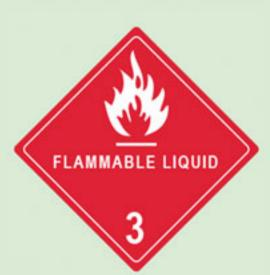
Steel drums and jerricans should meet DOT specifications and be in good condition. They will be marked with "UN 1A1" for steel drums and "UN 3A1" for steel jerricans. They must also be clearly labelled or marked to identify the fuel and the potential hazards e.g. gasoline - flammable.
